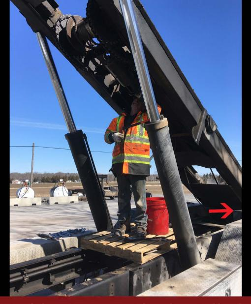
Safety blocks must be installed and designed to support the load before entering hydraulic supported components, including energy control procedures.
